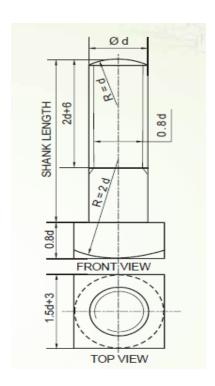
5. (Hint: Free hand sketch of stud with collar, d can be taken proportionately and calculate standard dimensions).
