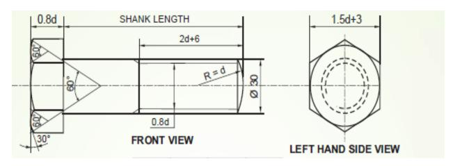
2. (Hint: Standard dimensions of BSW thread should becalculated with the pitch given = 30mm)
